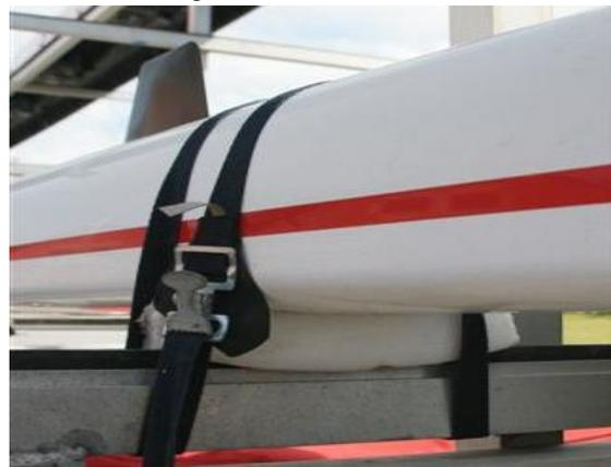
tighten the strap. The bow and stern deck are not designed for a heavy load and can be dented with too much pressure.
