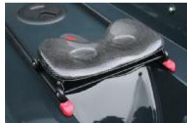
stern stops. And then slide the seat towards the bow making sure that the hooks of the seat riser are on the underside of the seat track flange. Sharply hit the stern end towards the bow to get the stern wheels over the stern stops. Once the seat is in the track, pull up on the seat to make sure it is properly in place. If one side pops up, remove and try again. If engaged properly, the seat should be able to hang from the seat tracks while upside down.
